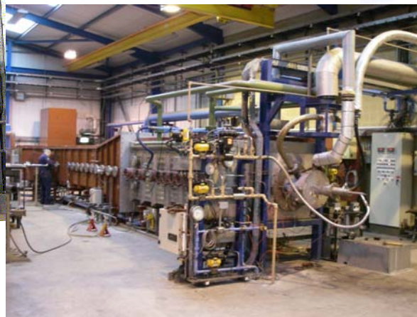
0.5 MW th Combustion Test Facility
